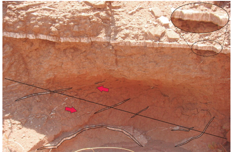
Figure 7. Picture showing the presence of fibrous gypsum-fillings in sigmoidal tensional fractures (indicated by the opposing arrows). By contrast, in the upper part a fibrous gypsum pseudobed fills a nearly horizontal fracture.
